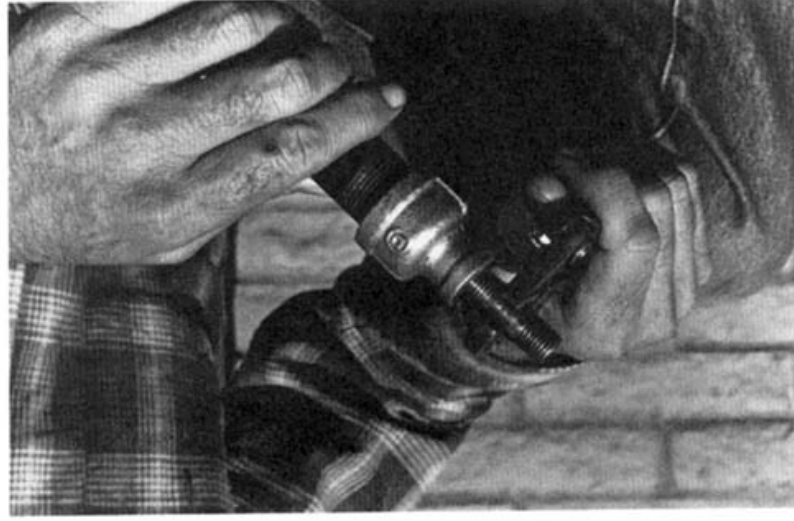
Then, using vise-grips, screw the 1/4 inch nipple into one of the reducers (as tightly as possible).
